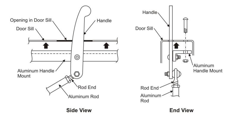
Note: Misalignment bushings are provided to make the handle and rod line up with the latch, if needed.
