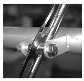
The supplied mounting tabs for the gas pedal are for mounting it from the dash bar. There are many other ways to mount the pedal which will require additional fabrication.
