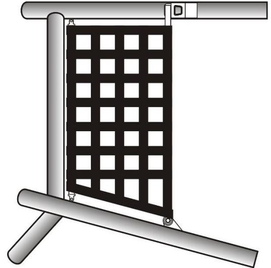
and tack the latch tongue to the chassis. Now tack weld the latch to the front net bar. Make sure the net opens and latches freely.
