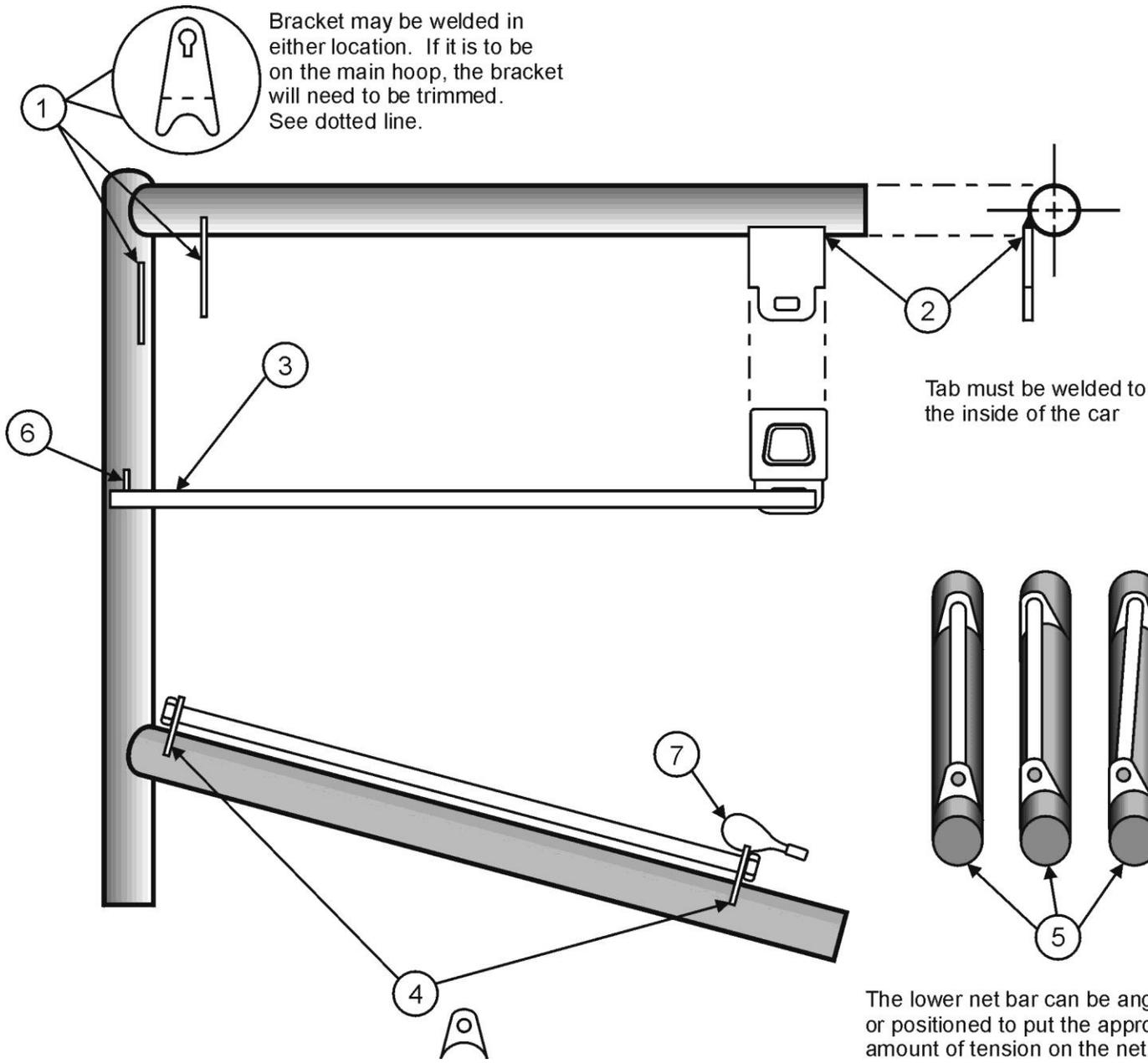
Bracket may be welded in either location. If it is to be on the main hoop, the bracket will need to be trimmed. See dotted line.
