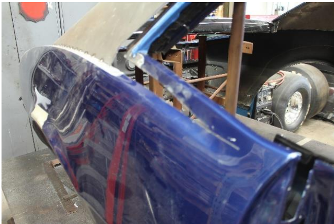
Wedge area cut out to move drip rail out
