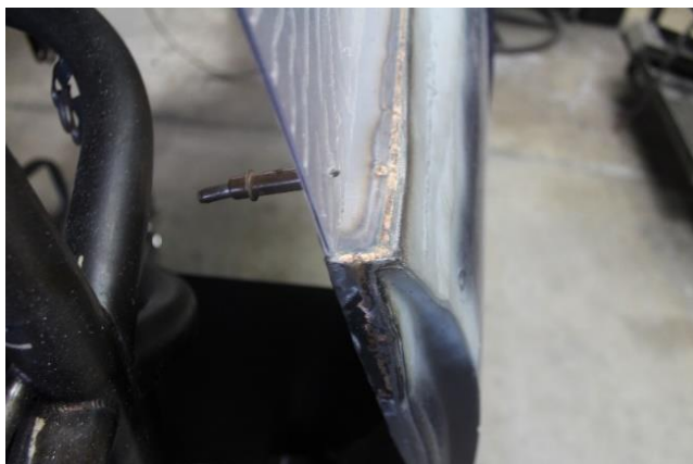
Window Support Welded into Place W/Lexan Cleco'd
