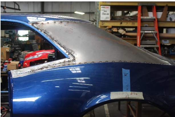
Panel & Wedge Tacked into Place – Outside
