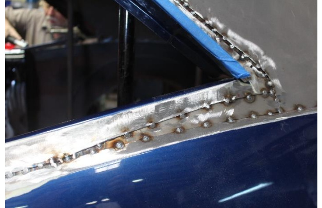
Side View – Wedge Tacked into Place
