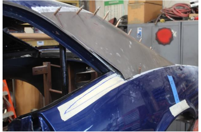
Frontside shows wedge area to be removed Allows drip rail to be pulled out to meet panel
